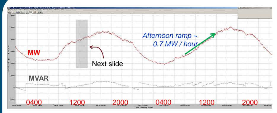
One-minute real & reactive power flow measured at distribution bus, 48 hour period
